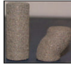
Figure 1. Porous nitinol ductility capacity under compression.
